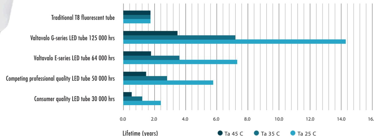
\*The graph is based on the Arrhenius equation commonly used in reliability analysis for electronics.
